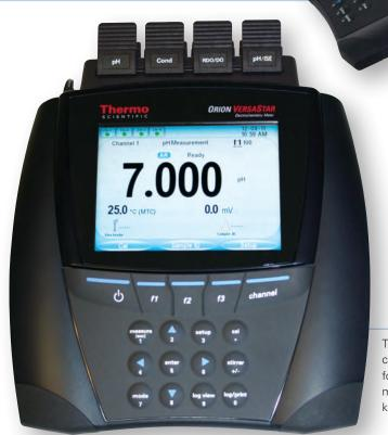
No need to turn off your meter to switch modules – meter automatically recognizes module changes.
