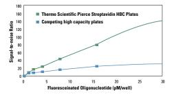
Comparison of Thermo Scientific Pierce Streptavidin High Binding Capacity (HBC) coated plate with competing high binding capacity plate. Plates were incubated with a biotinylated oligonucleotide, washed and probed with a complementary oligonucleotide labeled with fluorescein at various dilutions.
