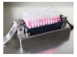
Tube racks, cluster, grid-referenced and twist-lock, polypropylene, Thermo Scientific Matrix SmartScan™
