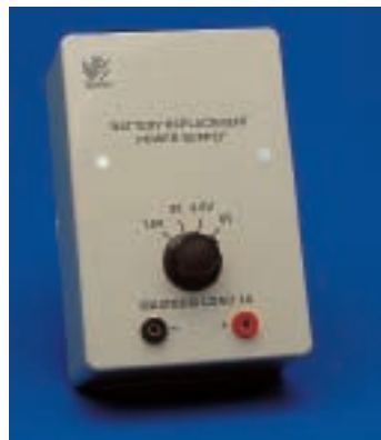
Power supply, battery replacement
