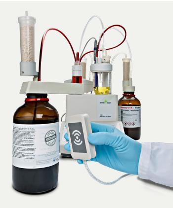
Our Hydranal™ bottles are embedded with an RFID chip, visible in the form of a new label, that captures essential information for every titration, including article code, product name, lot number, shelf life and numeric concentration.
