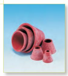
Sterilin Cones are for mounting filter funnels into Büchner flasks.
