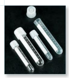
Sterilin Plastic Culture Tubes have a round base, suitable for suspension culture procedures.
