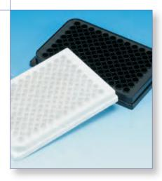
Sterilin black 96-well plates are for fluorescence work, and white plates are for bioluminescence studies.
