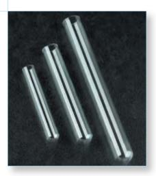
Sterilin Round Base, Rimless Borosilicate Glass Tubes are ideal for use with samples sensitive to leaching from plastic tubes.
